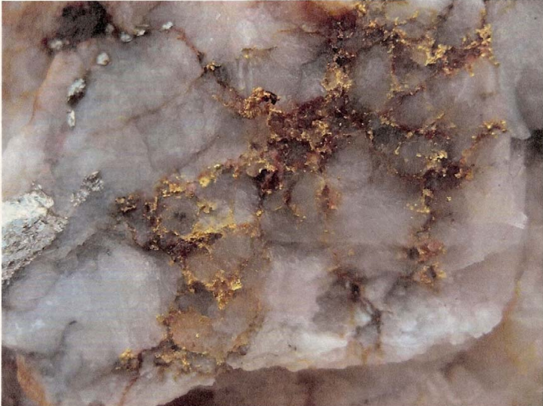
Gold Leaf – Golden Mile visible gold in grab sample #609954 grading 6,025 g/t Au (174 oz/t Au) Photo provided by Kodiak Exploration Limited
